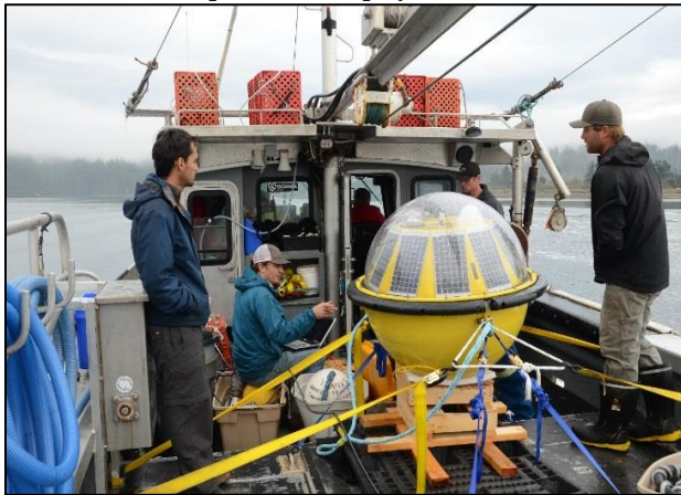
Figure 11: TRIAXYS buoy being transported to the measurement site in Port Renfrew
