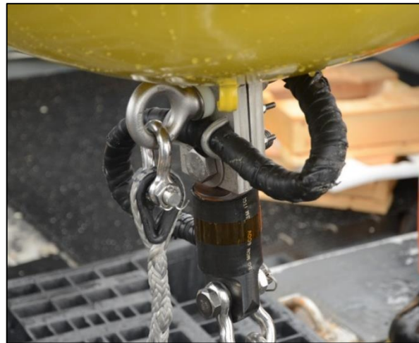
Figure 36: Connection between buoy and load cell
